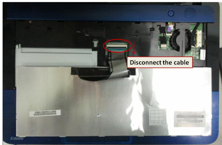
Figure 4-6-3 Disconnect the cable and remove the keyboard
